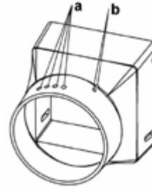
Install Keeper plate (item 108) on chute with one Tapping screw "T25 Torx drive" (item 142).
