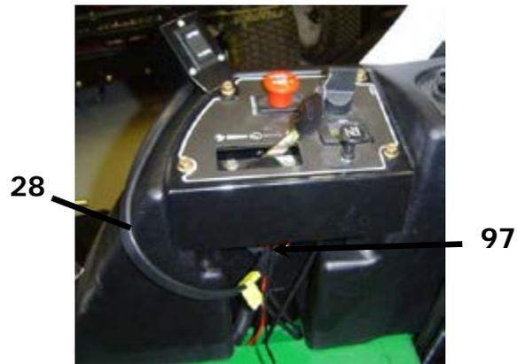
Route the **short** actuator connector (item a) wire to the back of the vehicle, from the **right side** of the vehicle.
