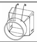
Install Keeper plate (item 108) on chute with one Tapping screw "T25 Torx drive" (item 142).
