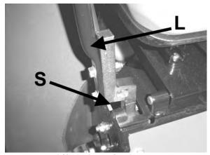
Lift and traction levers (operator's right side)
