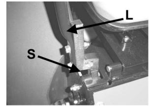
Lift and traction levers (operator's right side)
