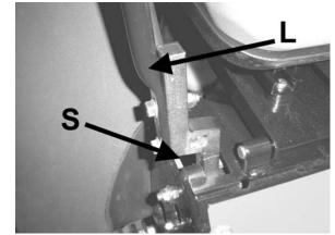
Lift and traction levers (operator's right side)
