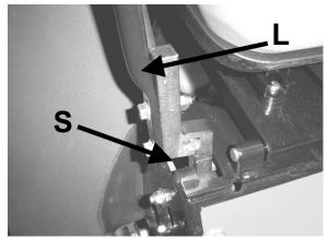
Lift and traction levers (operator's right side)
