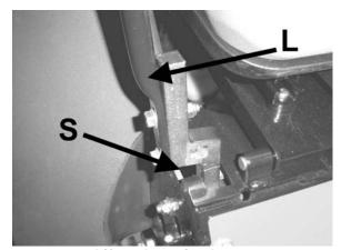
Lift and traction levers (operator's right side)
