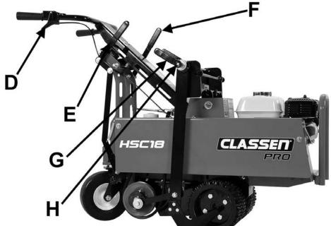
**THROTTLE (D)** - Squeeze the throttle control to increase the engine rpm. Squeezing the throttle control to increase the engine rpm also engages the centrifugal clutch powering the blades and wheels when the blades and/or wheel drives are engaged.
