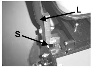
Lift and traction levers (operator's right side)
