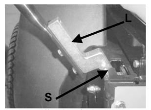
Lift and traction levers (operator's right side)
