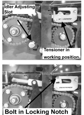
Bolt in Locking Notch Tensioning Position.
