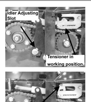
Bolt in Locking Notch Tensioning Position.
