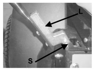
Lift and traction levers (operator's right side)
