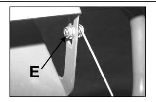
**NOTE:** Do not over tighten the chain. Excessive chain tension will reduce chain and bearing life. It can also lead to fatigue failure of the frame.
