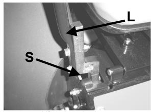
Lift and traction levers (operator's right side)
