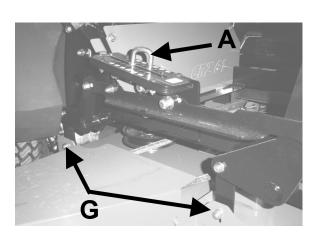
A 1/8" forward pitched deck provides the best horsepower. A level deck provides the best quality of cut. A 1/8" rearward pitched deck provides the best striping. Certain grass types and conditions may vary.
