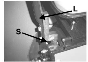
Lift and traction levers (operator's right side)
