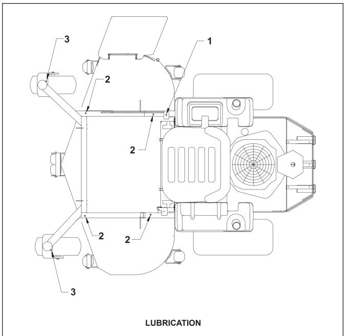
Every 50 hours of operation, lubricate the following points (1-3) with grease:
