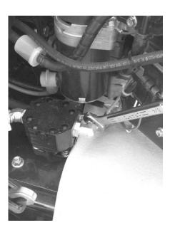
If the transaxles are noisy or jerky, purge the transaxles, following the purging procedures. See Purging Transaxles Page 9.
