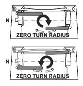
Slow down before making sharp turns. The machine is capable of turning very rapidly when the levers are moved further apart from each other. Loss of control and/or turf damage may result.
