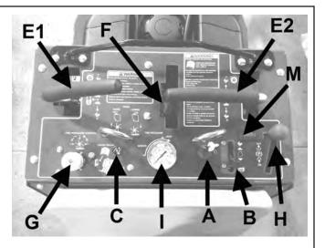
**RAISE-LOWER SWITCH (F)** - The raise-lower switch operates the hydraulics to raise and lower the tines. Rock the switch forward to lower the tines, rock it rearward to raise the tines.
