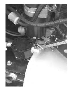
5. If the transaxles are noisy or jerky, purge the transaxles, following the purging procedures. **See Purging Transaxles Page 24**.
