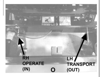
**MUD SCRAPERS(P)** - Mud scrapers for the drive wheels are provided. In ideal aeration conditions, soil should be moist but not so wet that it sticks to the tires.
