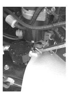
If the transaxles are noisy or jerky, purge the transaxles, following the purging procedures. See Purging Transaxles Page 24.
