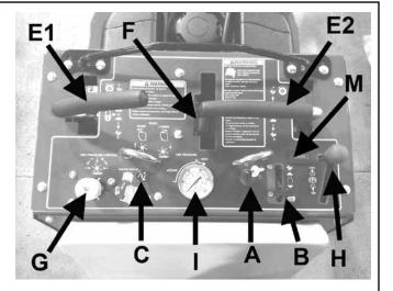
**RAISE-LOWER SWITCH (F)** - The raise-lower switch operates the hydraulics to raise and lower the tines. Rock the switch forward to lower the tines, rock it rearward to raise the tines.
