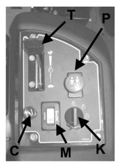
**THROTTLE (T)** - Move the throttle lever forward to increase engine speed until the maximum governed engine RPM is reached. Move the lever rearward to decrease engine speed until the engine reaches its idle speed.
