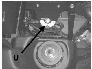
Located on oil cooler bracket behind seat.
