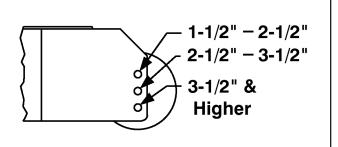
Height of cut ranges for roller adjustment
