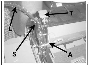
Lift and traction levers (operator's right side)
