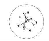
e) Loosen the jam nuts E on the height of cut clips F and adjusting screws G. Turn the adjusting screws G until the play is taken out of the chains H at all four corners. Tighten the jam nuts E against the clips F and at the adjusting screws G. Retighten nuts I at this time.
