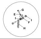
e) Loosen the jam nuts E on the height of cut clips F and adjusting screws G. Turn the adjusting screws G until the play is taken out of the chains H at all four corners. Tighten the jam nuts E against the clips F and at the adjusting screws G. Retighten nuts I at this time.
