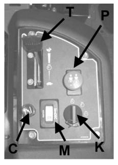
**THROTTLE (T)** - Move the throttle lever forward to increase engine speed until the maximum governed engine RPM is reached. Move the lever rearward to decrease engine speed until the engine reaches its idle speed.
