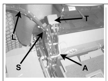
Lift and traction levers (operator's right side)
