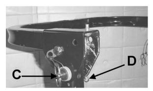
Remove cotter pin **D** from hitch pin **C**. Pull out hitch pin **C**, rotate upper hoop to the upright position. Reinstall hitch pin **C**. Reinstall cotter Pin **D** through hitch pin **C**.
