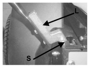
Lift and traction levers (operator's right side)
