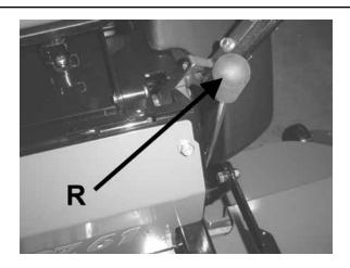
Parking brake in ON position (operator's left side)
