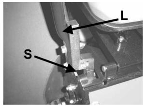
Lift and traction levers (operator's right side)
