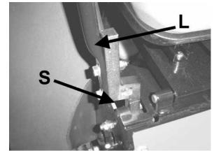
Lift and traction levers (operator's right side)
