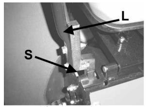
Lift and traction levers (operator's right side)
