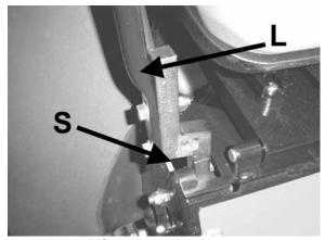
Lift and traction levers (operator's right side)
