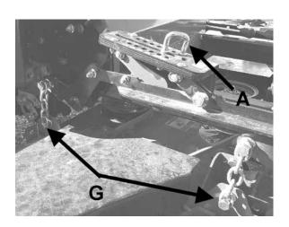
A 1/8" forward pitched deck provides the best horsepower. A level deck provides the best quality of cut. A 1/8" rearward pitched deck provides the best striping. Certain grass types and conditions may vary.
