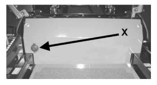
**Right Tank**: Fuel flows from the right tank when the selector is turned 1/4 turn toward the right.
