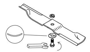
BLADE BOLT TORQUE: 70 FT-LBS (95 Nm)
