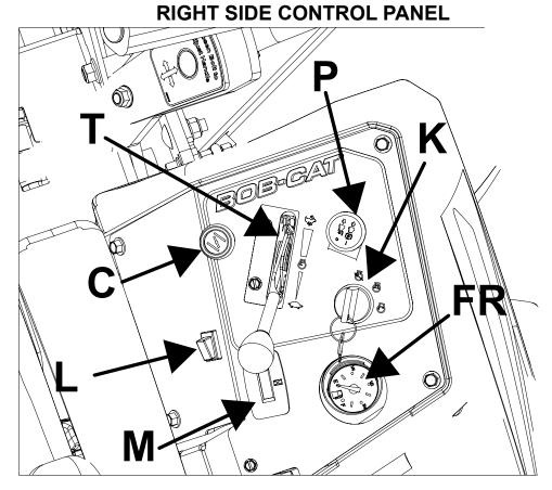
**THROTTLE (T) -** Move the throttle lever forward to increase engine speed until the maximum governed engine RPM is reached. Move the lever rearward to decrease engine speed until the engine reaches its idle speed.
