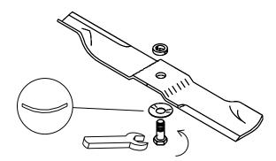
BLADE BOLT TORQUE: 70 FT-LBS (95 Nm)
