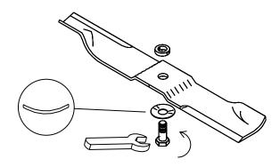
BLADE BOLT TORQUE: 70 FT-LBS (95 Nm)
