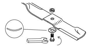
BLADE BOLT TORQUE: 70 FT-LBS (95 Nm)
