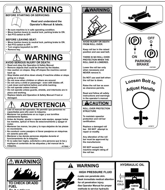
TO CHECK OR ADD FUEL -Do it outdoors. -Stop engine. Allow to cool. -Do not smoke. -Clean up spilled fuel. -Do not overfill. -Fill to one inch below bottom of filler neck. 2000570
