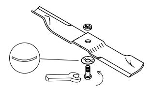
BLADE BOLT TORQUE: 70 FT-LBS (95 Nm)
