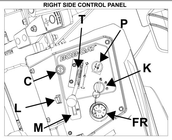
**THROTTLE (T) -** Move the throttle lever forward to increase engine speed until the maximum governed engine RPM is reached. Move the lever rearward to decrease engine speed until the engine reaches its idle speed.
