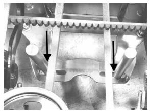
Adjust distance to 1/8" - 1/4" between deck drive belt and guides.
