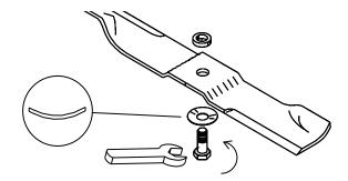
BLADE BOLT TORQUE: 70 FT-LBS (95 Nm)
