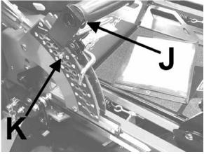
A 1/8" forward pitched deck provides the best horsepower.
