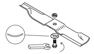
BLADE BOLT TORQUE: 70 FT-LBS (95 Nm)
