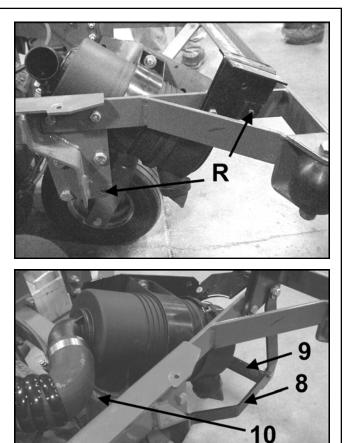
17. Slide the hose wrap 3 supplied in kit on the "S" shaped hose 5. Connect the air cleaner to the engine with the "S" hose and the (2) clamps from the Kohler Adapter/Elbow kit. The bend of the hose entering the engine should be horizontal. This allows the hose to clear the parking brake cable when the brake is off. Position the hose wrap to protect the hose from the parking brake cable when the parking brake is on.
