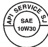
**NOTE:** Using other than service class SG, SH, SJ or higher oil or extending oil change intervals longer than recommended can cause engine damage. A logo or symbol on oil containers identifies the API service class and SAE viscosity grade.
