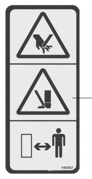
Moving blades/blade arms cut/crush Hazard
