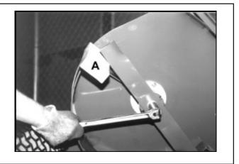
3. Remove blowout baffles A, mounting brackets B, and discharge baffle C. See **FIGURE A** for removal of these baffles. Retain baffles and hardware for conversion back to a side discharge deck.
