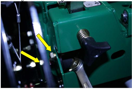
3) Put the seat back up, lift the foot pan. Take a 1/2" socket and 5/16" open end wrench and remove the nut from the ball socket of the control rod.
