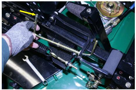
6) Take a flat blade chisel and hit the Push Nut sharply on the two areas where you see the tabs. The Push Nut should come right off if
