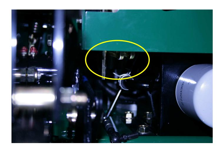
5) Remove two more cotter pins in the lift links. Note the outer link can be removed but the inner one requires the Lift Arm to slide partially out before it can be removed. (on reassembly to make it easier, just put the pin in from the other direction after the Lift Arm is installed)
