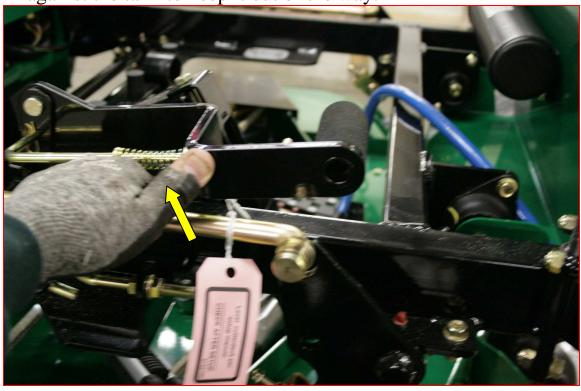
Now remove the Stovehead bolt (it needs to be removed for clearance
