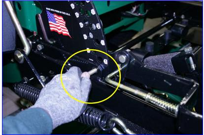
10) We can now remove the Lift Lever. With Foot lever folded out of the way start working the Lift Lever out. Note the inner link and pin will fall out once you move it a little. You may have to pull on the foot pedal to get it to clear the Lift Lever as well as put the control handle in the forward position off its slot and pull down on it as the ISO mount and control arm will interfere with it coming out.
