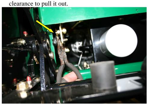
Once pin is removed and you have removed the control rod ball joint, put the ball joint up against the oil tank...this is important or it will get in the way during reassembly.
