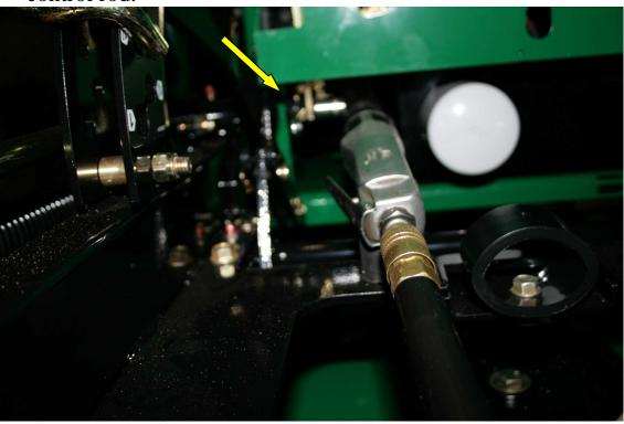
4) Take Needle nose pliers and remove <u>four</u> cotter pins – <u>one</u> in the pin of the reverse link. Remove the pin as well. Notice control rod is not yet removed. It is easier to remove it once you get the pin out as you can push the entire control arm assembly down and get
