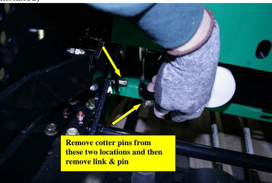
5) Remove the cotter pin from the inside of the spring loaded lift handle. And remove the assembly from the Lift Arm.
