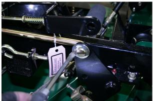
9) You need to get the lift rod out of the way. Push it out of the front hanger and while pulling out on the lift rod and pushing in on the Lift Lever, you can get them past each other. Pivot the lift rod up against the tank to keep it out of the way.
