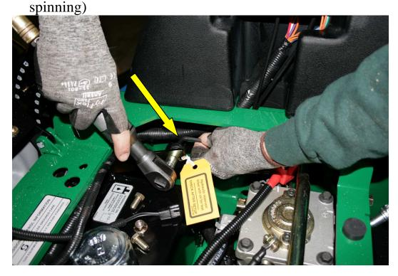
2) Use a 9/16 socket and 9/16 box end wrench to remove the two bolts
