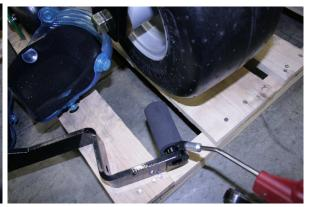
There is the possibility that normal "tolerance stack-ups" can result in a Lift Arm that will simply not clear the main frame (see below)
