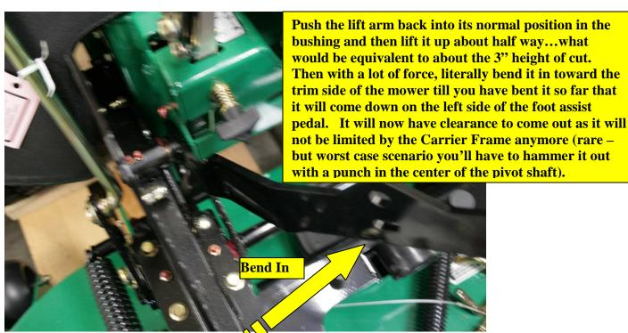
If this type interference occurs, you will have to use a rubber mallet to reinstall the new one as the main box will be contacting the new Lift Arm.
