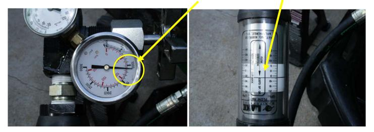
Take your reading, return the control lever to neutral, throttle back the engine and <u>open the Restrictor</u> <u>Valve all the way</u> in preparation for the wheel motor stall test. DO NOT DISCONNECT THE FLOW METER JUST YET.
