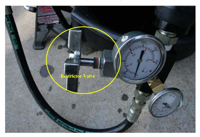
7. Put a jumper on the seat switch (or tie down operator presence bail on a walk-behind) and start the engine. Take it up to FULL throttle, and release the parking brake. Slowly stroke the control lever into forward, the wheel hub should be turning. (IF NOT, either you did not do Step 6 or your pump has totally failed)
