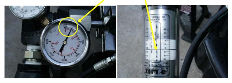
8. Continue turning the restrictor valve until it reaches 1100 PSI. Note the GPM again.
