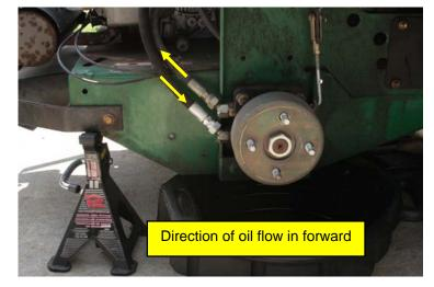
5. As long as you have a bi-direction meter with dual gauges you can remove either hose at the wheel motor. But if you only have one gauge like the meter shown below, *you will need to know which way the oil is flowing in the forward direction of travel so your gauge will read.* Typically with a single gauge like this, the oil has to flow into the side with the gauge.
