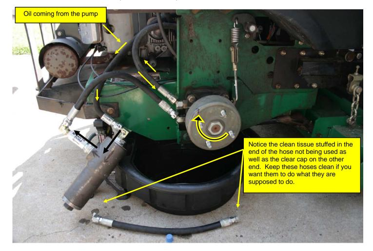
Notice the difference. The oil coming from the pump has to go through the filter first before it reaches the new wheel motor.
