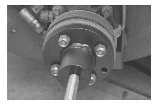
The 4 lug drum brake design uses four (4) of the 1/2-20 nuts, or you can use the existing lug nuts turned backwards.
