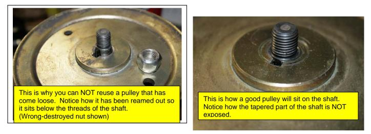
Once the nut comes a little loose, the pulley can rock. This eventually reams out the pulley as it runs. Fortunately the pump shaft is substantially harder than the pulley so the pulley takes most of the abuse. Typically little to nothing happens to the pump shaft. With extended running the key getting hammered in the keyway will take the most abuse. See the following pictures for example of what you can expect to find.
