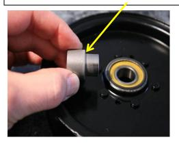
This is wrong. Shoulder on spacer is not seated tight against bearing race.
