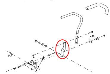
**Action Required:** Due to possible breakage of 4168100 Control Bar, it must be replaced with kit 4170482 S-Control Bar Assembly. The distributor will ship the appropriate number of kits to the dealer to cover all units purchased (refer to Products Involved section below).
