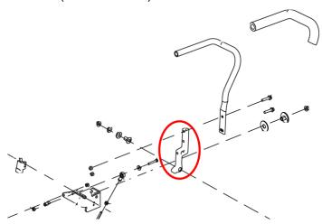
**Action Required:** Due to possible breakage of 4168100 Control Bar, it must be replaced with kit 4170482 S-Control Bar Assembly. The factory will ship the appropriate number of kits to the dealer to cover all units purchased (refer to Products Involved section below).
