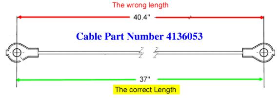
**Action Required:** If the reel does not engage when the bail is pulled back, remove the side cover guard, measure the cable length, and replace the cable if it measures 40.4 inches long.
