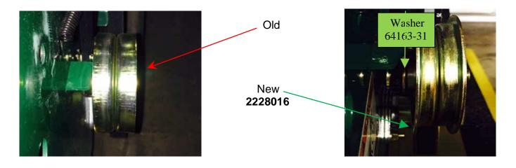
**Action Required:** Units in the below affected serial range, need a pulley 2228016 with washer 64163-31 installed in place of existing pulley (548942).
