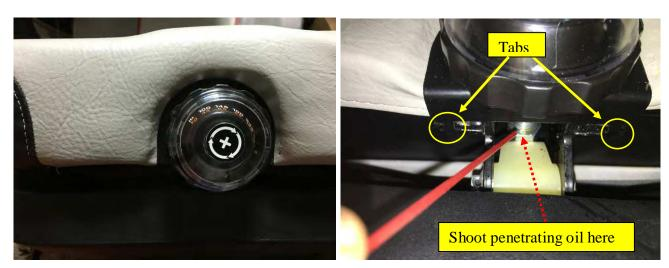
Units that have this style adjusting knob, have a rubber skirt at the front of the seat. The rubber skirt is simply held on by two metal tabs. Push the skirt back and shoot penetrating oil on the adjuster bolt as shown in the picture above.
